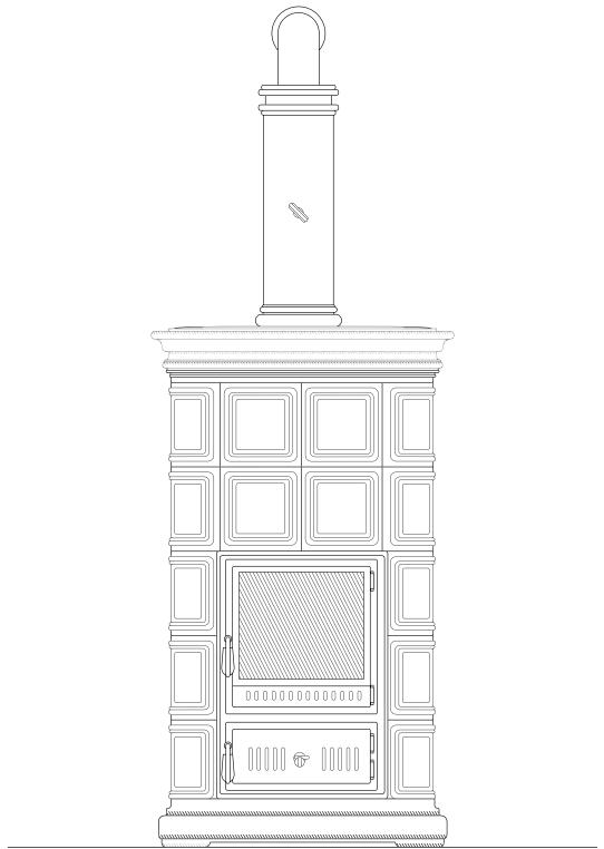
— Eng [L/A] — Wood-burning with additional accumulation. This collection of stoves harks back to Nordic tradition, both in its geometry and in the decorative painting of the “tiles” pattern of graphic and minimal effect on the exterior. They are designed to be installed freely anywhere, without the support of a wall.
